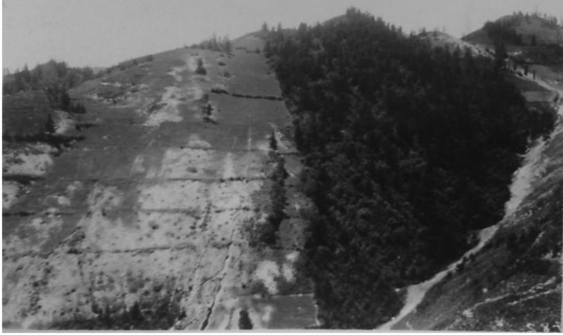
IMAGE 2. Dongzhai study area: “‘Contrast Valley,’ showing a remnant of the former natural forest and shrub vegetation and the results of slope cultivation. Superficial run-off plots in pairs were located within the forest and on two phases of the cultivated and denuded portion of the slope.” Walter C. Lowdermilk Papers, Hoover Institution Archives, box 9.
